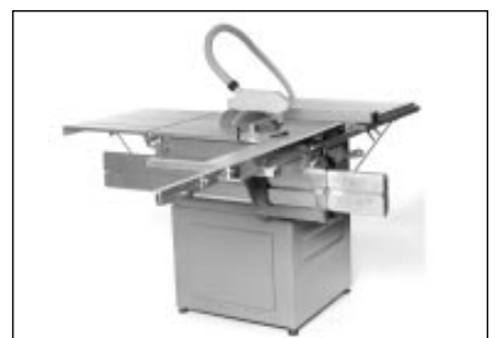
Pull sliding carriage back. Turn work around by 180°, swing flipstop down again and place squared edge against the stop. Make second cut.
